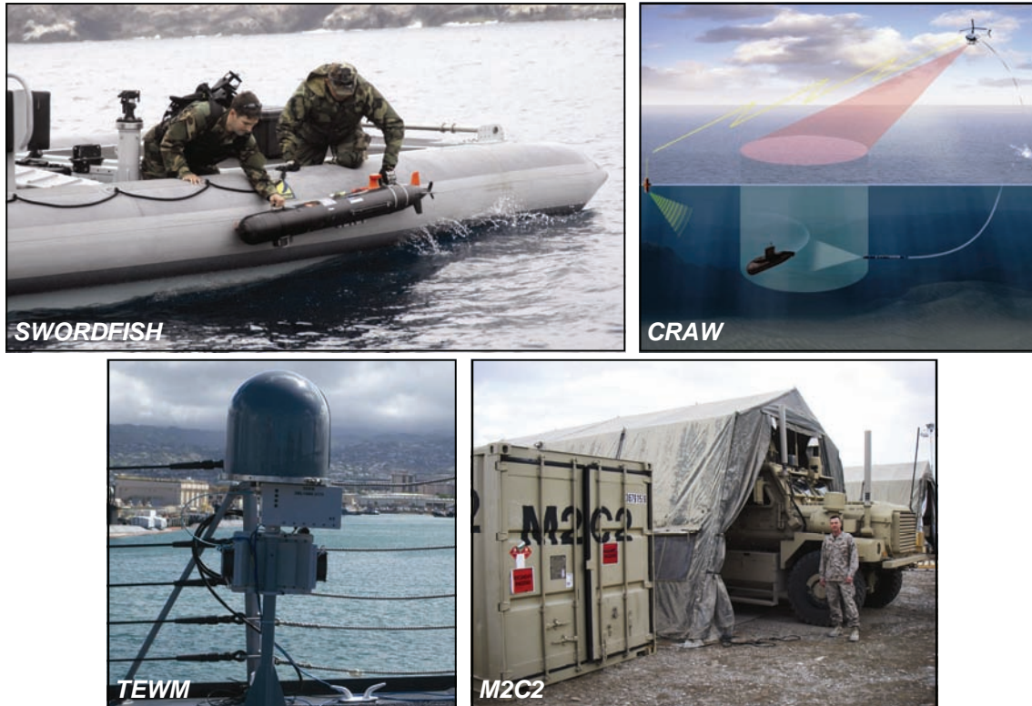
Examples of Speed to Fleet projects that provide initial capabilities to the Fleet/Force: The MK 18 MOD 1 SWORDFISH is a small (two-person portable), low-cost UUV, for U.S. Navy Explosive Ordnance Disposal Forces; the Compact Rapid Attack Weapon (CRAW) is a lightweight anti-submarine torpedo designed to be deployed from the Fire Scout Unmanned Aerial Vehicle; the Transportable Electronic Warfare Module (TEWM) installed on USS Sampson during RIMPAC 2010 provides surface ships a layer of protection from kinetic and non-kinetic attack; and the U.S. Marine Corps Mobile Modular Command & Control Vehicle (M2C2) provides command and control elements with efficient, broadband connectivity for voice and data communications.
